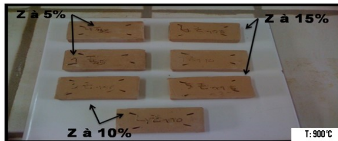
Photo.1. Color of fired bricks at 900°C, after doping with various percentage of Al_2O_3 .
