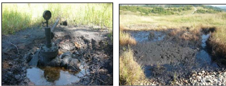
Fig. 9 –GPS.259 point: Oil derrick for hydrocarbon extraction - points of primary production in the G sector (left) and GPS.309 point: Oil spot (areas affected by crude oil discharged from the extraction source) next to the 309 Oil derrick in the I sector (right) (Photo source: Florin Vartolomei)
