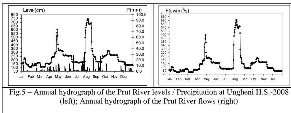
Fig.5 – Annual hydrograph of the Prut River levels / Precipitation at Ungheni H.S.-2008 (left); Annual hydrograph of the Prut River flows (right)
