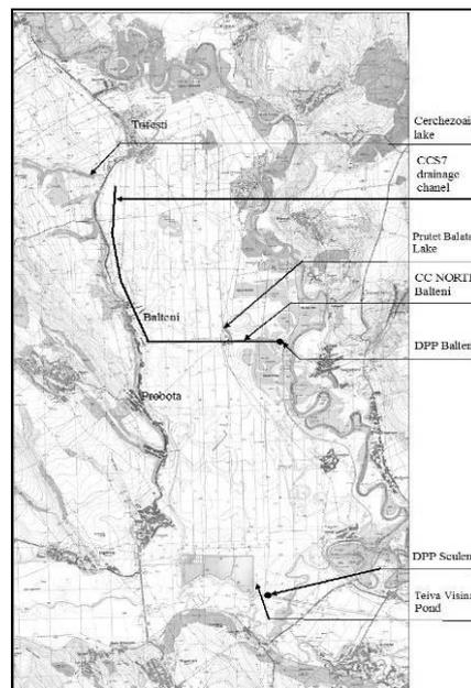
Fig. 8 – Trifești Sculeni embankment enclosure; draining channels; evacuation of excess of water in the Prut and Jijia Rivers
