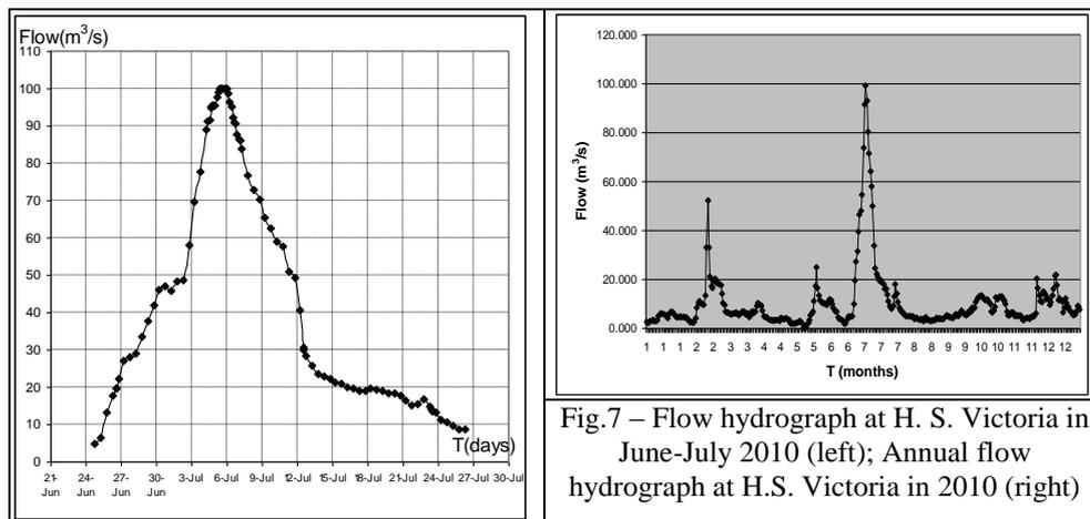
Fig.7 – Flow hydrograph at H. S. Victoria in June-July 2010 (left); Annual flow hydrograph at H.S. Victoria in 2010 (right)
