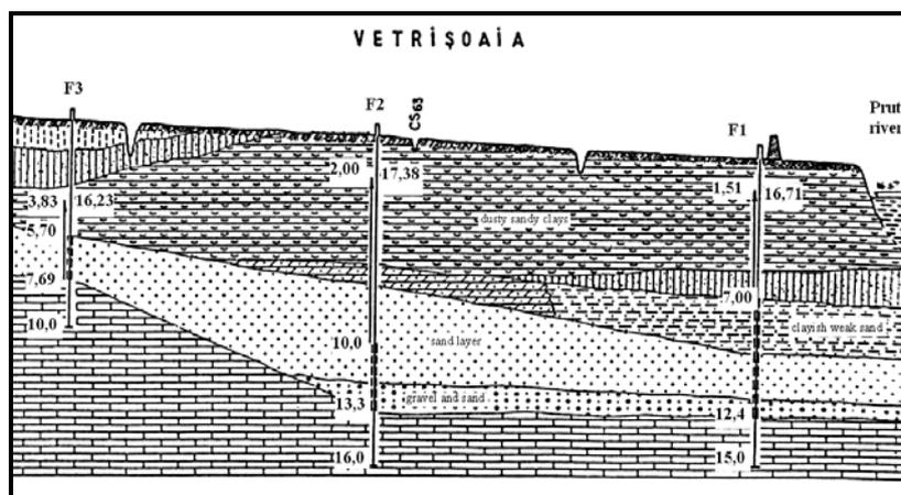
Fig. 3 - Hydrogeological profile
