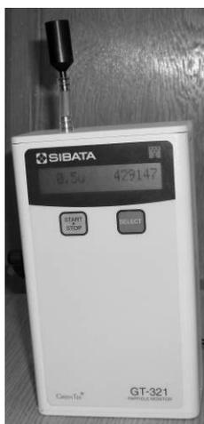
Fig. 1 - Optical particle counter SIBATA GT 321
