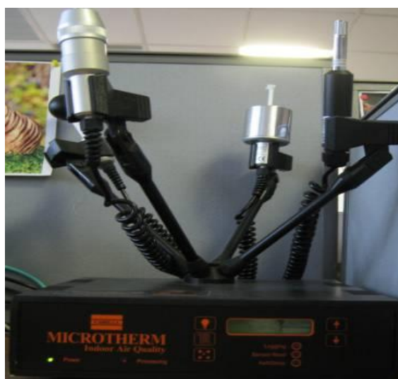
Fig. 3 - Casella MicroTherm – Indoor Climate System
