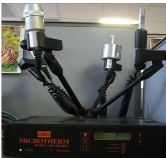
Fig. 3 - Casella MicroTherm – Indoor Climate System
