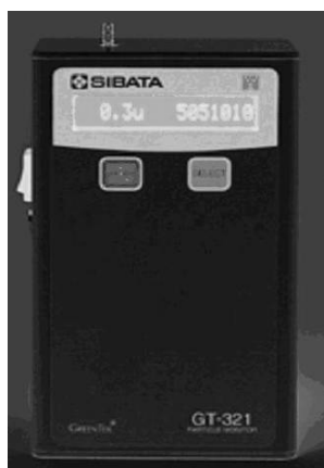
Fig. 8 - SIBATA GT 321 – the particle counter
