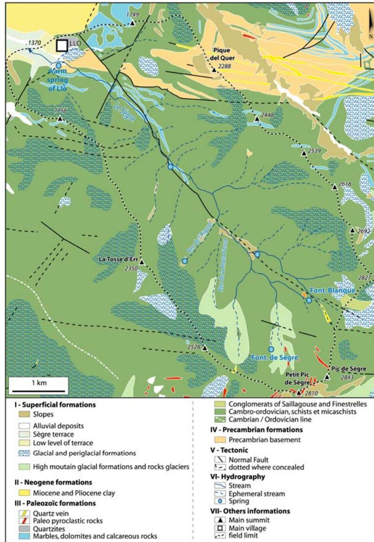
Fig. 1 - Geologic extract of the 1/50000th card (map) Saillagouse, redrawn and simplified
