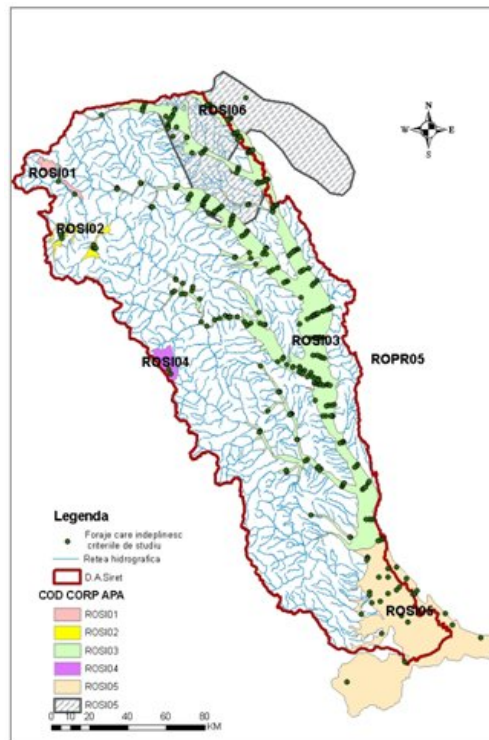
Fig. 3. Map of drillings remaining after achievement steps and criteria presented, on the basis of which have established the Natural Background Levels (NBL) and Threshold Values (TV's) for each groundwater body from Hydrographical Siret Basin
