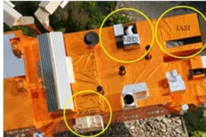
Fig. 2 - The display of instruments on the board of METOP-A satellite
