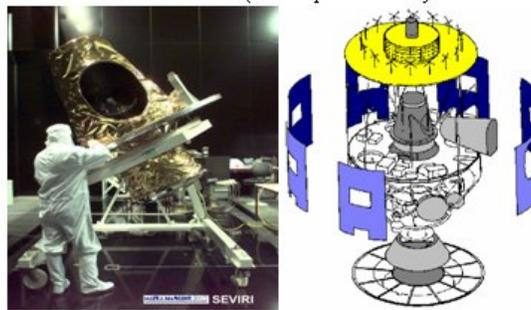
Fig. 1 - Spinning Enhanced Visible and Infrared Imager
