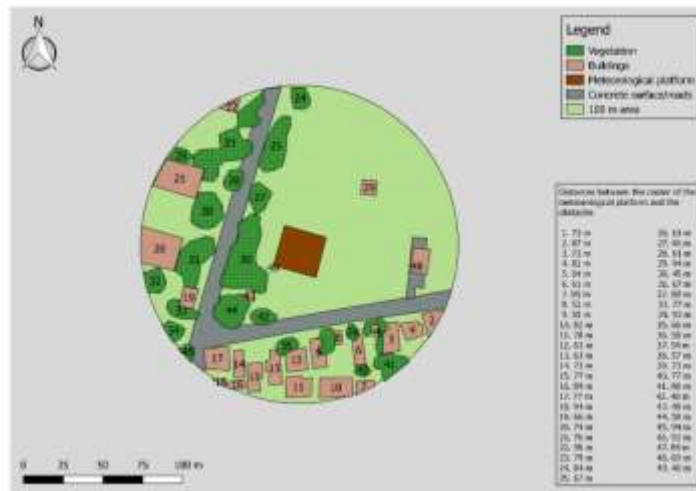
Fig. 2 – The obtained image with the vectorized obstacles for Iași meteorological station using Qgis software package
