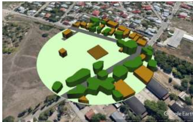
Fig. 4 – The obstacle image with the vectorized obstacles for Iași meteorological station transposed in 3D using Google Earth
