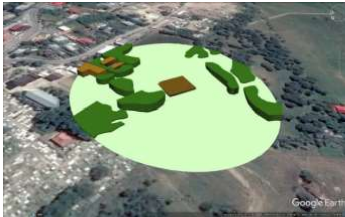
Fig. 3 – The obstacle image with the vectorized obstacles for Botoșani meteorological station transposed in 3D using Google Earth
