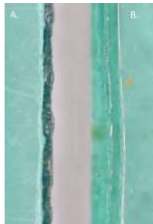
Figure 4. Cutting method comparison: a. guillotine cut (left) vs. b. laser cut (right)
