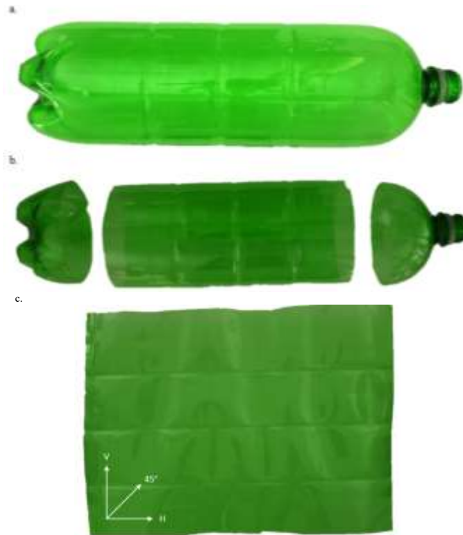
Figure 3. a. Complete Bottle, b. Top and Bottom Removed and c. Curled Flat Sheet
