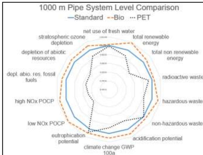
Fig. 5. Pipe System Level Comparison
