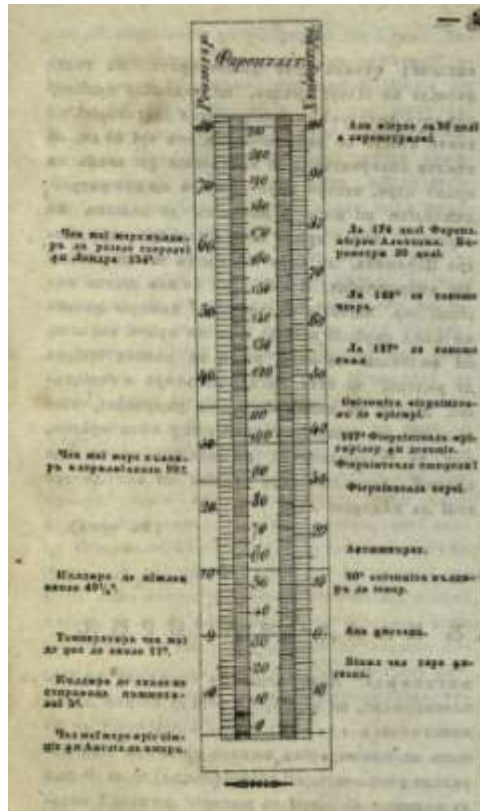
Fig. 3. Thermometer depicted in “Icoana lumii”, 1841, with scales in Réaumur, Fahrenheit, and Celsius (source: National Digital Library of Romania)
